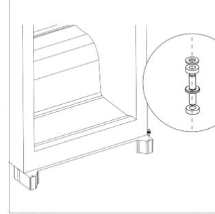
7. Unscrew top hinge pin from the hinge. Then turn the hinge over and screw hinge pin.
