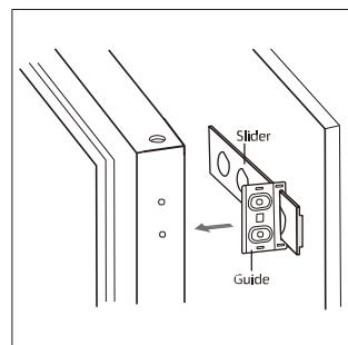
7. Fit two guides with sliders and fix them with short screws.
