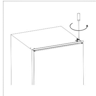
2. Unscrew bottom hinge of freezer door. Then remove the door and place it on a soft pad to avoid scratch.
