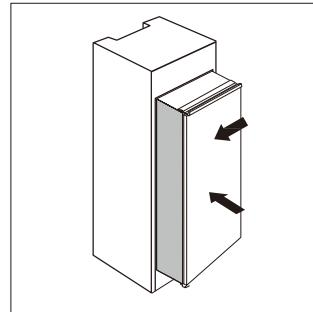
3. Screw a guide to holes in the side of appliance door with short screws.
