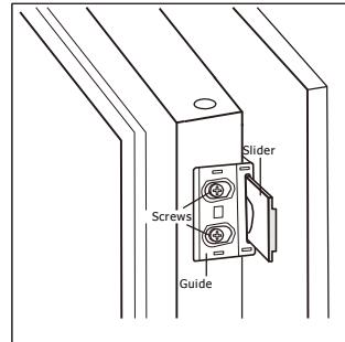
4. Open the appliance door and the wooden door together. Once the door opens and closes at all angles, mark the position of the slider. Take slider out of guide and fix slider with wooden door by two short screws. Then fix slider cover onto the slider.
